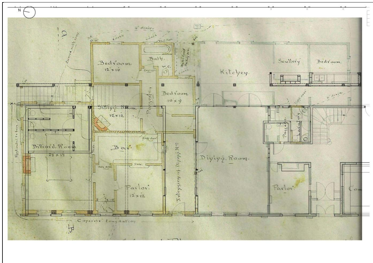
Figure 5: Plan of the rebuilt structure overlaid onto the original plans of the Messenger extension
