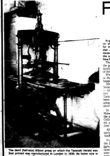
The demi (half-size) Albion press on which the Taranaki Herald was first printed was manufactured in London in 1830. Its home now is in the Taranaki Museum in New Plymouth.
